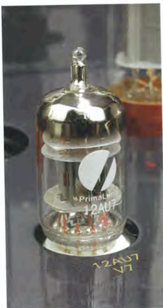
At front sit six 12AU7 preamplifier valves, small-signal double triodes.
